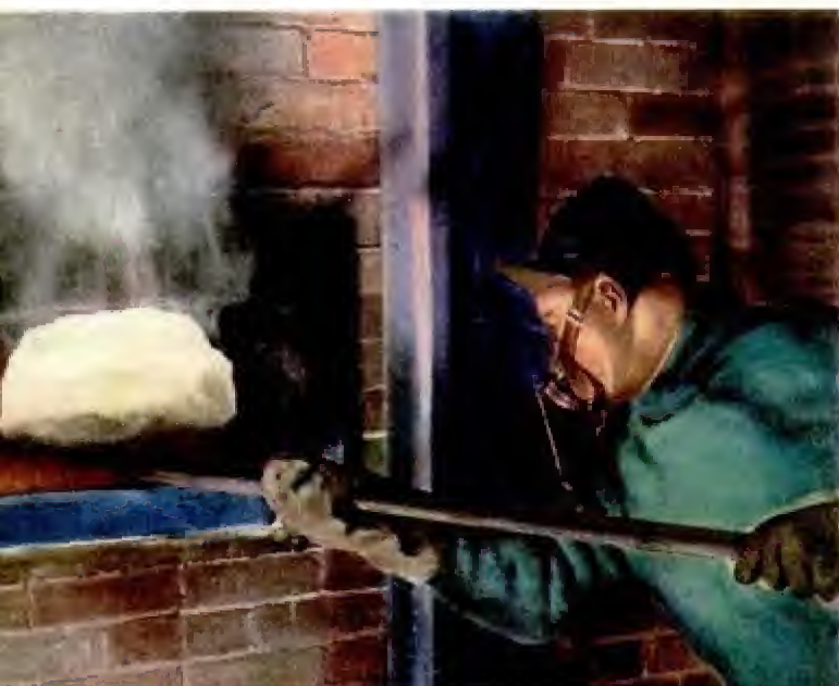
The first step in refining radium, as in treating many other ores, is to roast out impurities in the furnace. This is a scene at Eldorado refinery, Port Hope, Ont.
